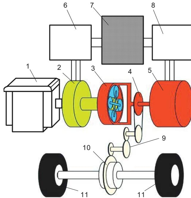
Fig. 1.23. Power train of Toyota Prius hybrid electric vehicle (HEV): 1 — gasoline engine, 2 — PM brushless generator/starter (GS), 3 — power split device (PSD), 4 — silent chain, 5 — PM brushless motor/generator (MG), 6 — GS solid state converter, 7 — battery, 8 — MG solid state converter, 9 — reduction gears, 10 — differential, 11 — front wheels.
