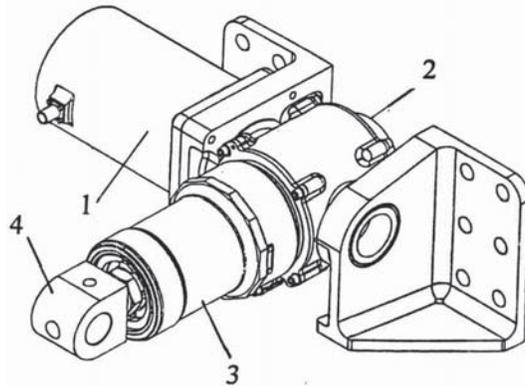
**Fig. 1.24.** Electromechanical actuator for flight control surfaces: 1 — brushless motor, 2 — gearbox, 3 — ball lead screw, 4 — clevis or spherical joint end.
