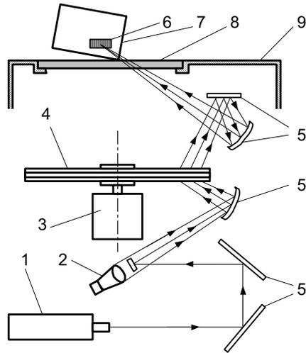
**Fig. 1.16.** Bar code scanner: 1 — laser, 2 — photodecoder converting laser beam into electric signal, 3 — PM brushless motor, 4 — holographic three-layer disk, 5 — mirror, 6 — bar code, 7 — scanned object, 8 — scan window, 9 — housing.
