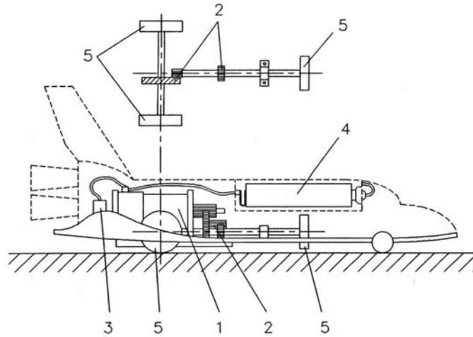
**Fig. 1.18.** Toy space shuttle: 1 — PM d.c. commutator motor, 2 — transmission, 3 — on-off switch, 4 — 1.5-V battery, 5 — driven wheels.
