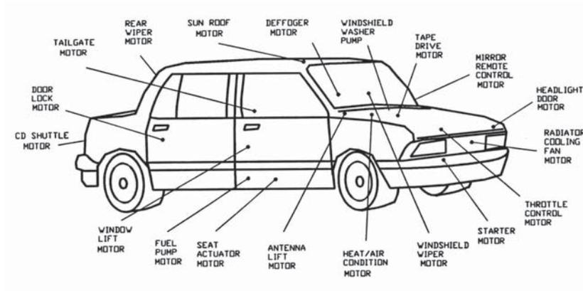
Fig. 1.22. PM motors installed in a car.
