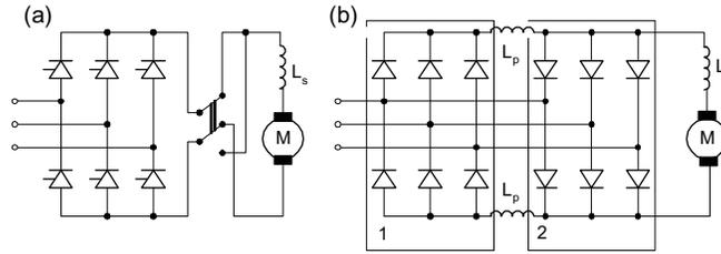
**Fig. 1.2.** d.c. commutator motor drives: (a) one quadrant, fully-controlled, single-converter drive, (b) four-quadrant, fully-controlled, dual converter drive;  $L_p$  are reactors limiting the currents circulating between the rectifying and inverting bridges,  $L_a$  is the armature circuit inductance.
