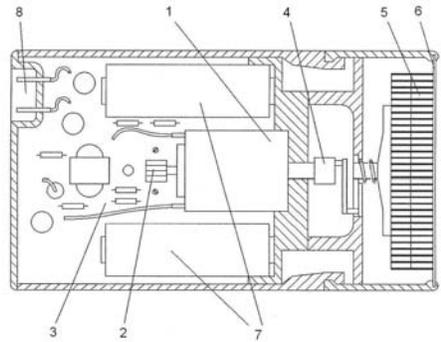
**Fig. 1.17.** Electric shaver with a PM brushless motor: 1 — PM brushless motor, 2 — position sensor, 3 — printed circuit board, 4 — cam-shaft, 5 — twizzer head, 6 — platinum-coated shaving foil, 7 — rechargeable battery, 8 — input terminals 110/220 V.
