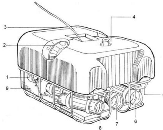
**Fig. 1.30.** Underwater robotic vehicle for remote inspection of hydro power plants: 1 — two thruster sets for forward and reverse (200-W d.c. brushless motors), 2 — two thruster sets for lateral and vertical (200-W d.c. brushless motors), 3 — buoyancy material, 4 — transponder, 5 — flood light, 6 — still camera, 7 — video camera, 8 — electric flash, 9 — cover. Courtesy of Mitsui Ocean Development and Eng. Co., Tokyo, Japan.
