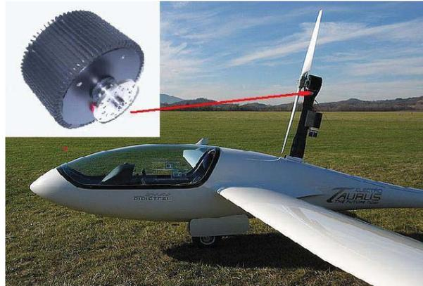
**Fig. 1.27.** *Taurus Electro* two-seat self launching glider with a 30 kW, 1800 rpm, 15.8 kg PM brushless motor. Photo courtesy of Pipistrel, Ajdovscina, Slovenia.
