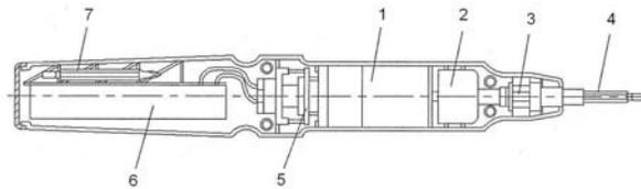
**Fig. 1.28.** Cordless electric screwdriver: 1 — PM d.c. commutator motor 3.6 V/240 mA, 2 — speed reducer, 3 — locker for manual screwing, 4 — screwdriver bit, 5 — forward-reverse rotation switch, 6 — rechargeable Ni-Cd battery, 7 — bit compartment.
