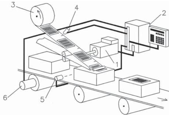
**Fig. 1.15.** Automatic labelling systems with a PM brushless motor: 1 — PM brushless motor servo drive, 2 — controller, 3 — spool of self-adhesive labels, 4 — registration mark sensor, 5 — box position sensor, 6 — conveyor speed encoder. Courtesy of *Parker Hannifin Corporation*, Rohnert Park, CA, U.S.A.
