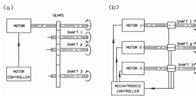
**Fig. 1.31.** Gear train design: (a) conventional system, (b) mechatronics system.
