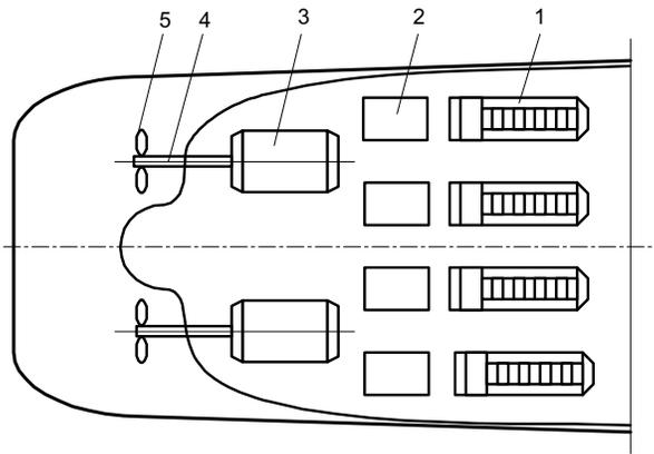
**Fig. 1.25.** Ship propulsion system with a PM brushless motor: 1 — diesel engine and synchronous generator, 2 — converter, 3 — large PM brushless motor, 4 — propeller shaft, 5 — propeller.
