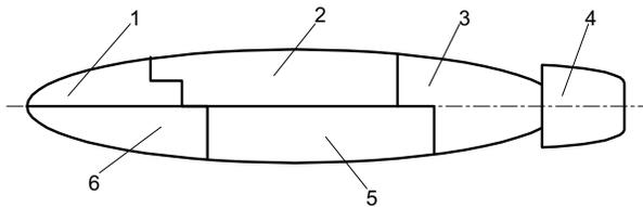
**Fig. 1.26.** Stealth torpedo: 1 — guiding system, 2 — conformal acoustic arrays, 3 — advanced rechargeable batteries, 4 — integrated PM brushless motor propulsor, 5 — active and passive noise control, 6 — synergic drag reduction.
