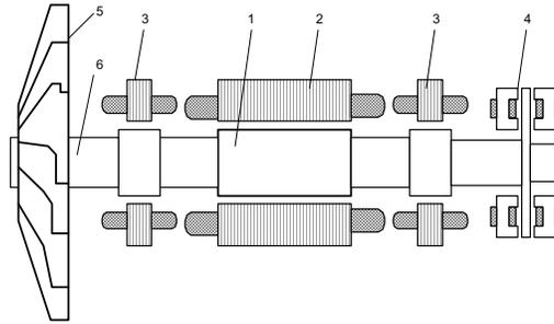
**Fig. 1.14.** Centrifugal chiller compressor with high speed PM brushless motor and magnetic bearings: 1 — rotor with surface PMs and nonmagnetic can, 2 — stator, 3 — radial magnetic bearing, 4 — axial magnetic bearing, 5 — impeller, 6 — shaft.
