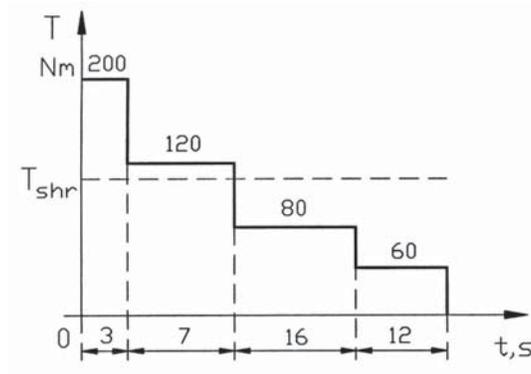
**Fig. 1.35.** Torque profile of the electric motor. *Numerical example 1.2.*
