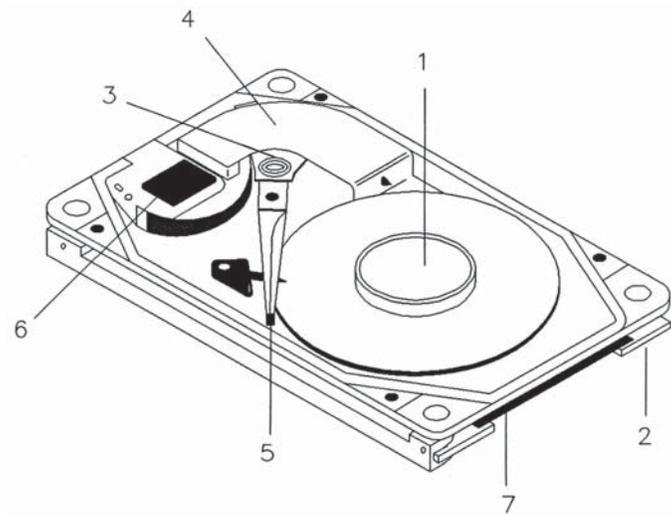
**Fig. 1.20.** Computer hard disk drive (HDD) with a PM brushless motor: 1 — in-hub PM brushless motor mounted in 2.5-inch disk, 2 — integrated interface/drive controller, 3 — balanced moving-coil rotary actuator, 4 — actuator PM, 5 — read/write heads, 6 — read/write preamplifier, 7 — 44-pin connector.
