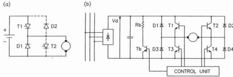
**Fig. 1.3.** Chopper controlled d.c. motor drives: (a) one-directional with added regenerative braking leg, (b) four-quadrant chopper controller [167].
