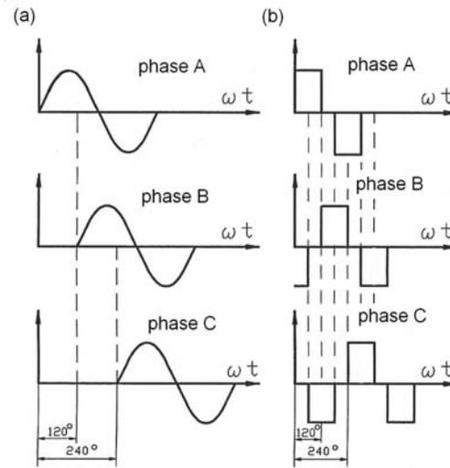
**Fig. 1.1.** Basic armature waveforms for three phase PM brushless motors: (a) sinusoidally excited, (b) square wave.
