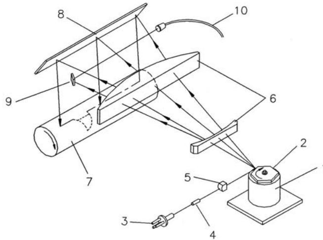
**Fig. 1.21.** Laser beam printer: 1 — stepping motor, 2 — scanner mirror, 3 — semiconductor laser, 4 — collimator lens, 5 — cylindrical lens, 6 — focusing lenses, 7 — photosensitive drum, 8 — mirror, 9 — beam detect mirror, 10 — optical fiber.
