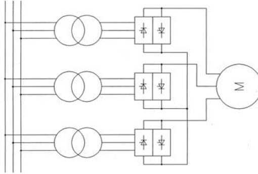
**Fig. 1.5.** Cycloconverter synchronous motor drive.
