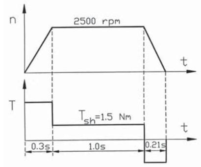
**Fig. 1.36.** Speed and torque profiles of a servo drive. *Numerical example 1.3.*
