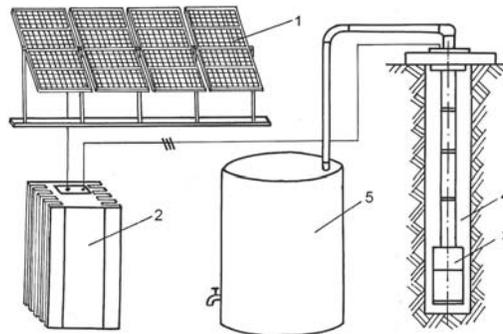
**Fig. 1.29.** Water pumping system for a remote population center: 1 — solar panels, 2 — inverter, 3 — submersible PM brushless motor-pump unit, 4 — well, 5 — water storage tank.
