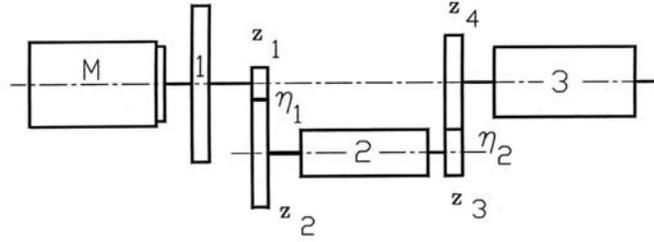
**Fig. 1.34.** Electric motor driven rolling mill. *Numerical example 1.1.*
