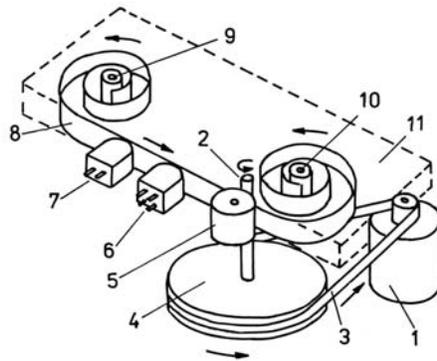
**Fig. 1.19.** Cassette deck: 1 — PM motor, 2 — capstan, 3 — belt, 4 — flywheel, 5 — pressure roller, 6 — rec/play head, 7 — erase head, 8 — tape, 9 — supply reel table, 10 — take-up reel table, 11 — cassette.
