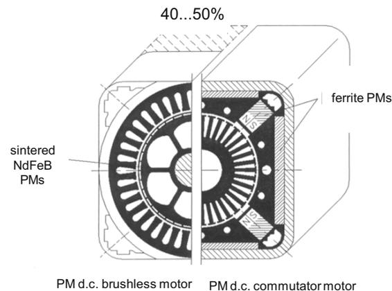
**Fig. 1.11.** Comparison of PM brushless and PM d.c. commutator motors.
