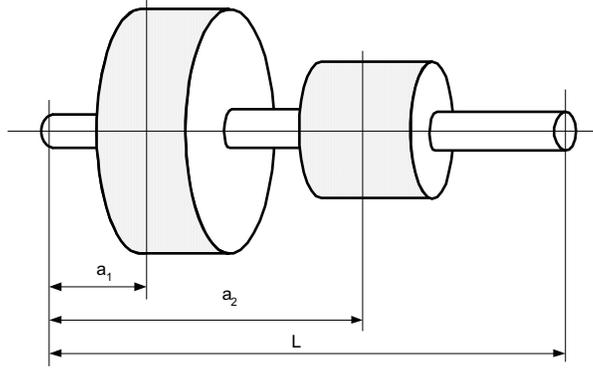
**Fig. 1.33.** Solid cylindrical shaft loaded with two masses  $m_1$  and  $m_2$ .
